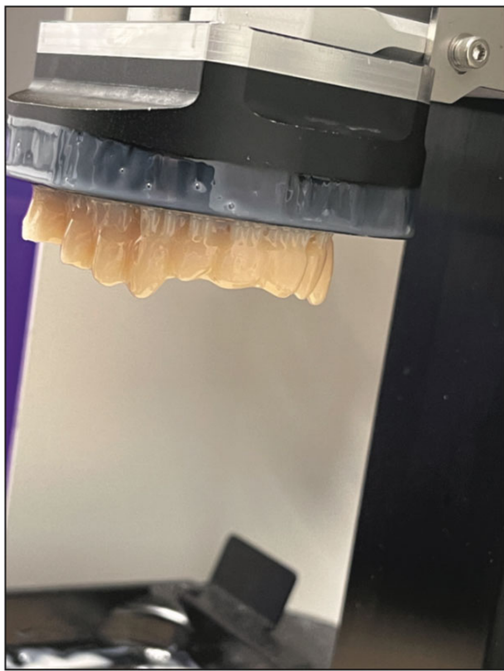
Figure 8. The second temporary bridge was printed in Rodin Sculpture on the SOL 3D printer (Ackuretta).
